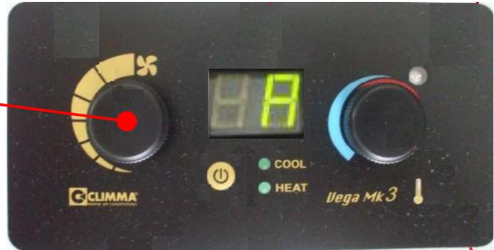
**Important note:** if the functioning mode AF- Auto-special is selected, the fan speed range is automatically limited. In COOL mode the minimum speed is #5 in auto and #3 in manual. In heat mode the minimum speed is #3. In heat mode, if the HP safety stops the compressor, at restart the speed is rised by 2 steps both at first and at the second intervention. At third intervention the system is locked out.
